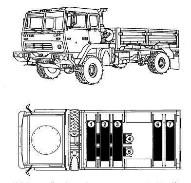
Figure 10-21b. Loading the truck, cargo, LMTV, LVAD/AD, 2<sup>1</sup>/<sub>2</sub> ton, M-1081.
