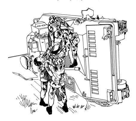
Figure 8-35. BIFV driver evacuation, vehicle on side.
