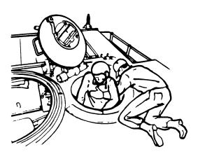
Figure 8-32. Loader's hatch opening.
