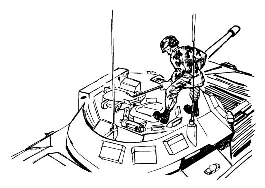
Figure 8-36. Opening gunner's hatch from outside vehicle.
