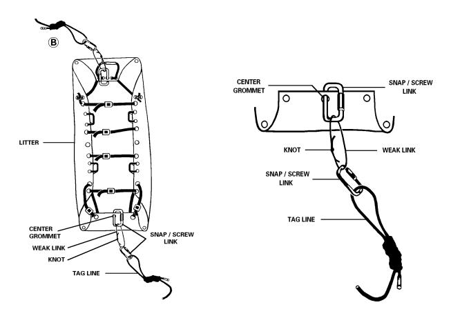
Figure E-2. Connection of the weak line to SKED litter and tag line (continued). (B—Alternate method of using center grommet.)
