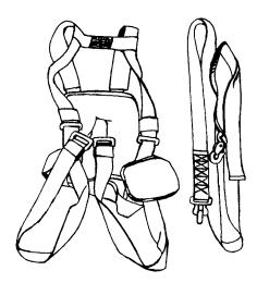
Figure E-1. Vest, hoist operator, and lifeline.
