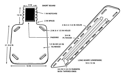
Figure 9-16. Prefabricated spine boards (short and long).
