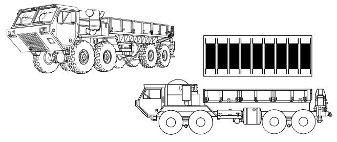
Figure 10-18. Heavy expanded, mobility tactical truck, 8x8, cargo, M977.
