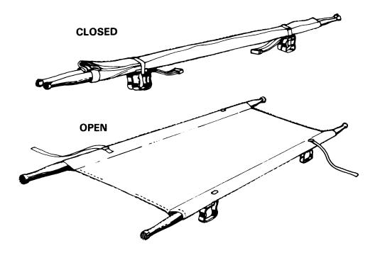
Figure 9-1. Standard collapsible litter.
