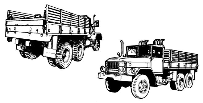
Figure 10-17. Truck, cargo, 5 ton, 6x6, wide bed, and truck, cargo, 21/2 ton, 6x6, wide bed.
