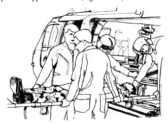
Figure 10-30. Loading litter into UH-60A.
