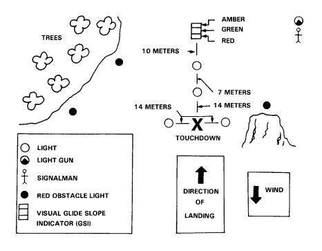
Figure 10-28. Field expedient inverted landing zone (night).
