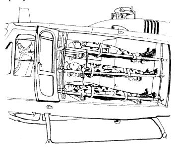
Figure 10-32. Interior view of UH-1H/V Iroquois six-litter configuration.
