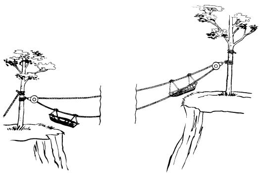
Figure 9-29. Evacuation by horizontal hauling line.
