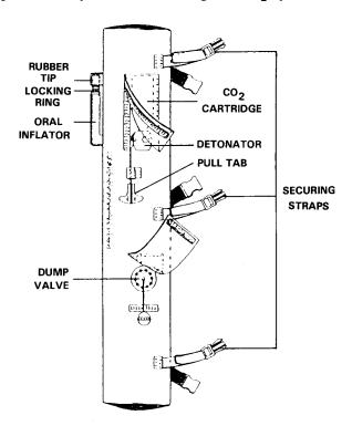
Figure E-8. Inflating the flotation log.
