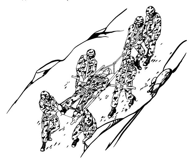
Figure 9-27. Modified travois (descending steep slope).
