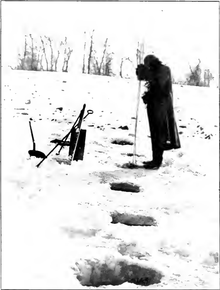
Winter Gauging of Southferk River near Cowley, Alta. Taken by P. M. Sauder.
